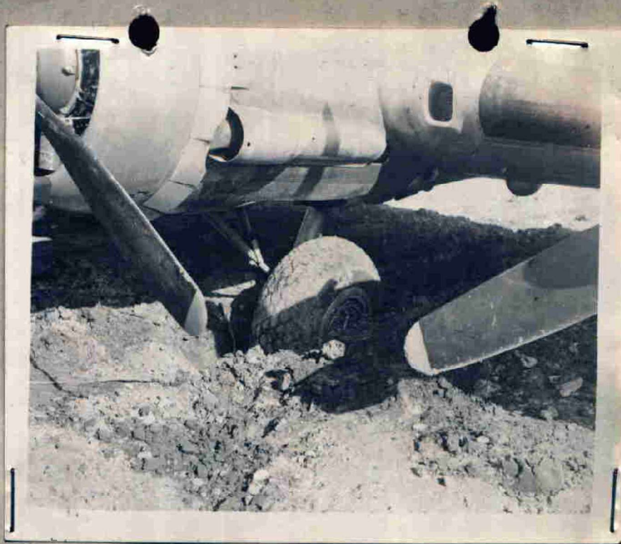
Top views shows a close up shot of the left front wheel after the pilot had run into a soft spot on the new taxing strip that had just been finished. Bottom view shows the reward of quick thinking on the part of the pilot in cutting the switches on engines #1 and #2, no damage to the propellers.
