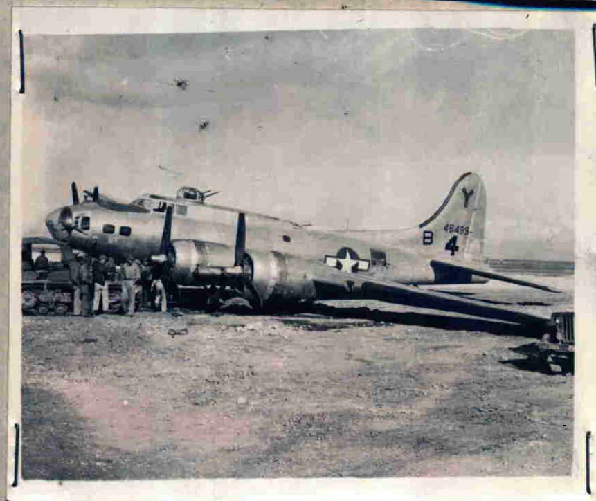
Top views shows a close up shot of the left front wheel after the pilot had run into a soft spot on the new taxing strip that had just been finished. Bottom view shows the reward of quick thinking on the part of the pilot in cutting the switches on engines #1 and #2, no damage to the propellers.
